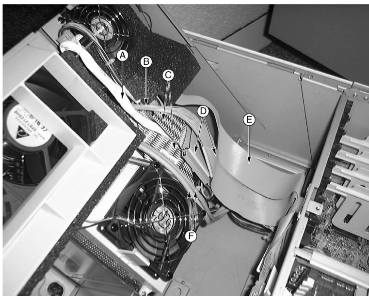
Figure 9 - Cables to the subchassis
